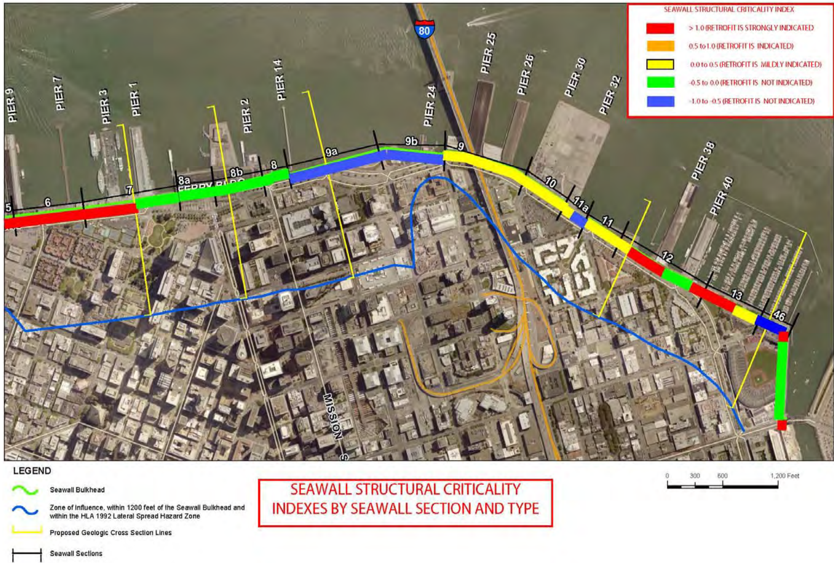
Figure 4-54: Bulkhead Wall Structural Criticality Ratings by Location, Section 6 to Section China Basin
