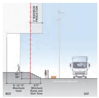
FIGURE 5.8 - Working Waterfront Zone - Elevated Walkway condition
