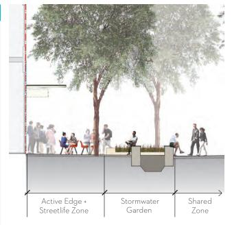
FIGURE 4.2.3 Section at Stormwater Garden
