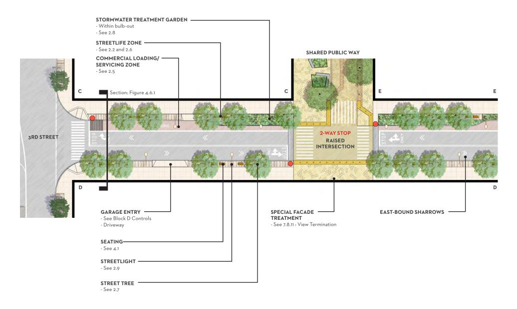
**FIGURE 4.6.2** Long Bridge Street Conceptual Plan. This is provided for illustrative purposes only & does not represent a design proposal. Refer to Chapter 8 of the Infrastructure Plan for key dimensions, intersection analysis, and fire access information.
