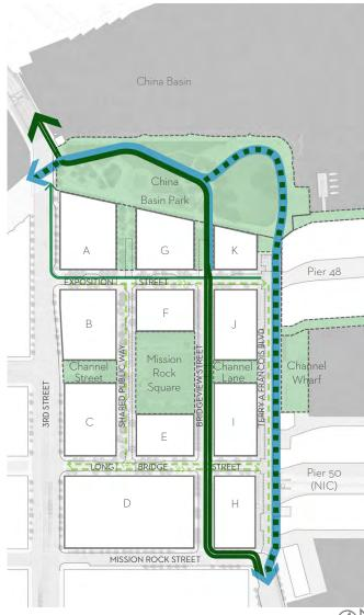
FIGURE 2.4.2 Bicycle Circulation Network Diagram illustrating hierarchy and connections among the different types of bicycle facilities across the site. These facilities are described in Chapters 3 and 4 for each open space and street.
