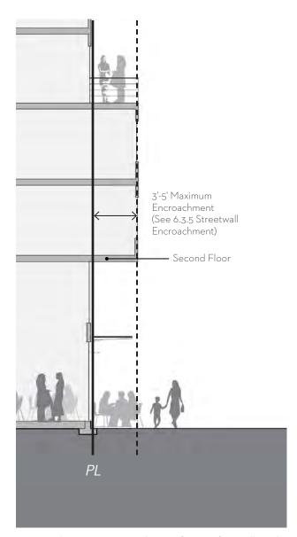
On typical streets, an encroachment of up to 3 feet is allowed, starting at the second floor and above.
