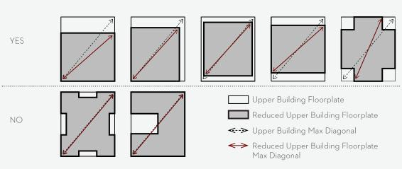
FIGURE 6.4.7 - Examples of Floorplate Reduction
