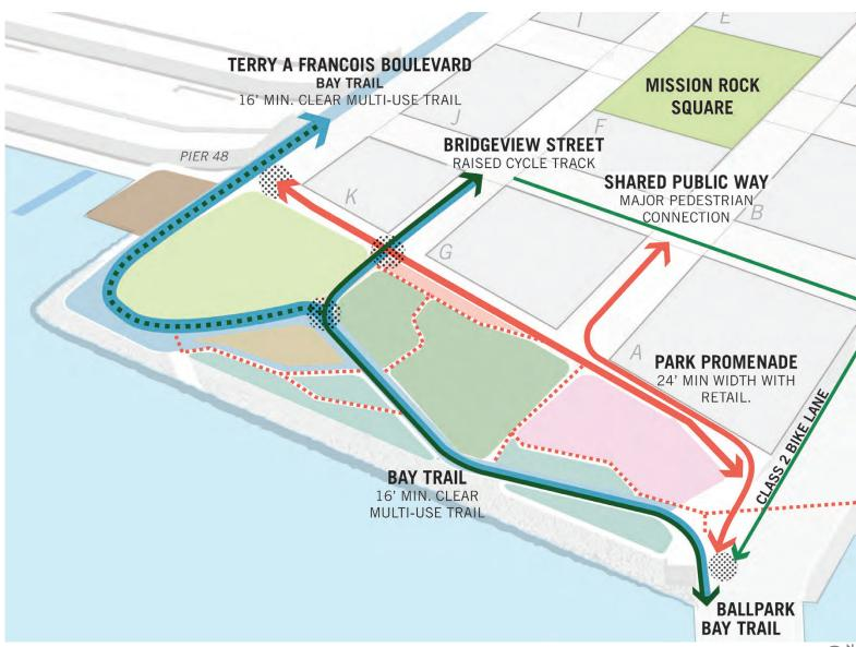
**FIGURE 3.2.3** Circulation + Connections: This diagram illustrates the circulation connections described in Standards 3.2.7-3.2.9, including the Bay Trail/Blue Greenway, a major pedestrian and bicycle route; the Park Promenade, a pedestrian-only connection; and secondary, smaller-scale paths. These will connect important site anchors such as Pier 48, the Shared Public Way and Mission Rock Square, and the Ballpark.
