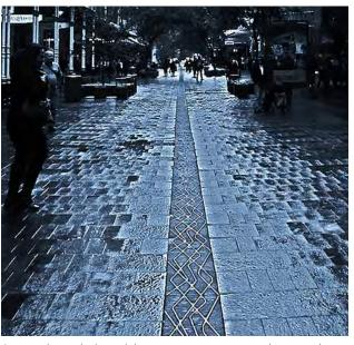
A special trench drain delineates uses or zones within a single field of paving. Source Newtown Graffitti / FLICKR
