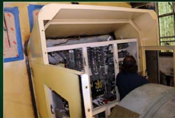
Carbody slope is attached and additional work is being done on the low-volt wiring system.
