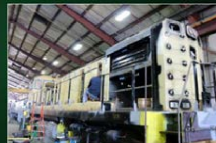
Carbody and panels are installed and radiator is welded in place.
