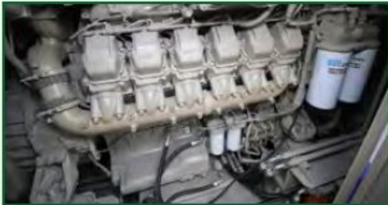
The MTU engine used in the SE10B is approximately half the size of the engine it typically replaces.
