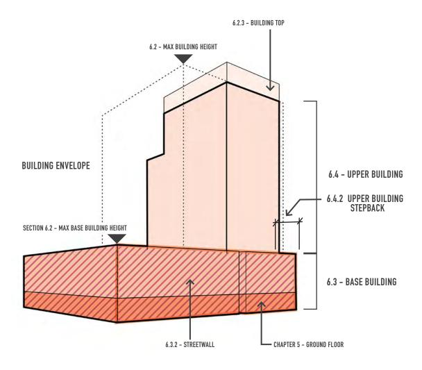
FIGURE 6.1 - Components of the Building Envelope
