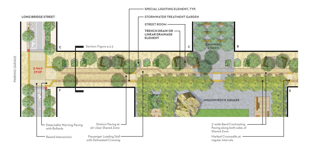
FIGURE 4.2.4 Shared Public Way Conceptual Plan that satisfies the controls herein. This is provided for illustrative purposes only and does not represent a design proposal. Refer to Chapter 8 of the Infrastructure Plan for key dimensions, intersection analysis, and fire access information.
