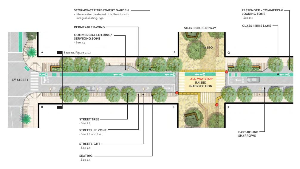
FIGURE 4.5.2 Exposition Street Conceptual Plan. This is provided for illustrative purposes only & does not represent a design proposal. Refer to Chapter 8 of the Infrastructure Plan for key dimensions, intersection analysis, and fire access information.
