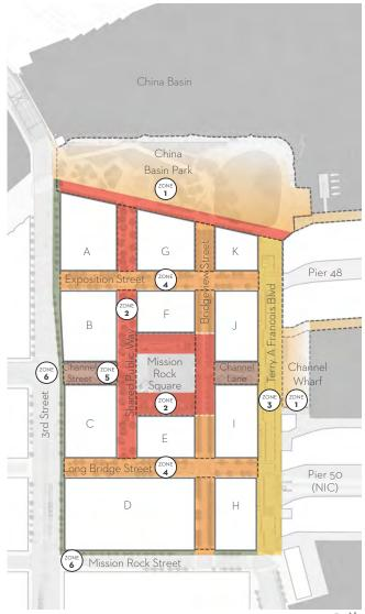
FIGURE 2.9.2 Lighting Zones Diagram illustrating the distribution of lighting zones described in Figure 2.9.1.
