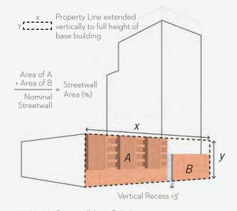
FIGURE 6.3.2 - Streetwall Area Calculation
