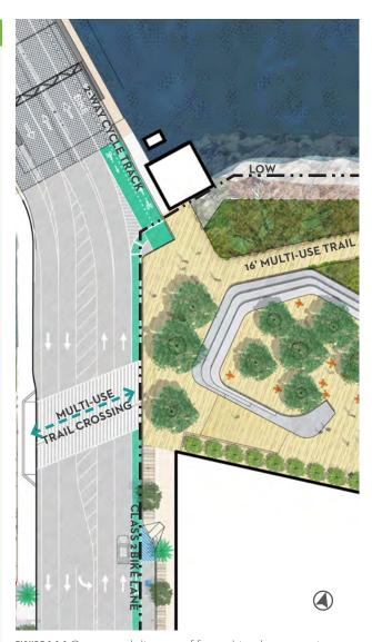
**FIGURE 3.2.2** Conceptual diagram of future bicycle connections at Lefty O'Doul Bridge that satisfies the controls herein. This is provided for illustrative purposes only and does not represent a design proposal.
