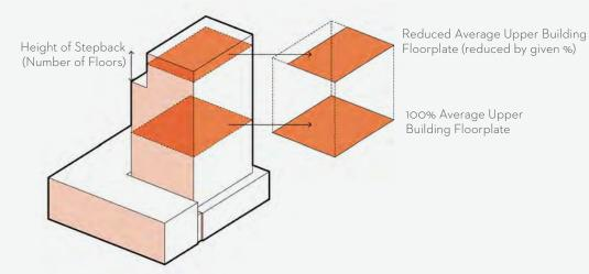
FIGURE 6.4.6 - Floorplate Reduction
