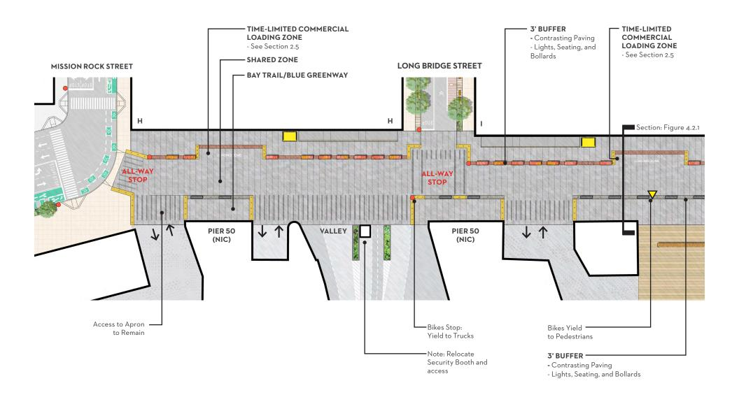
FIGURE 4.3.2 Conceptual Plan of Terry A Francois Boulevard. This is provided for illustrative purposes only & does not represent a design proposal. Refer to Chapter 8 of the Infrastructure Plan for key dimensions, intersection analysis, and fire access information.
