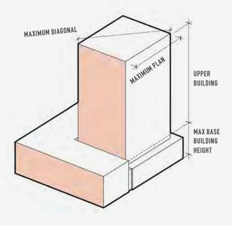
FIGURE 6.4.4 - Maximum Plan Length and Diagonal Length
