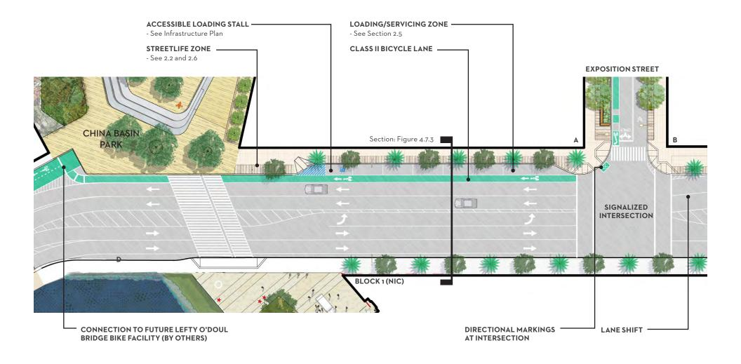
**FIGURE 4.7.2** 3rd Street Conceptual Plan at Block A. This is provided for illustrative purposes only & does not represent a design proposal. Refer to Chapter 8 of the Infrastructure Plan for key dimensions, intersection analysis, and fire access information.
