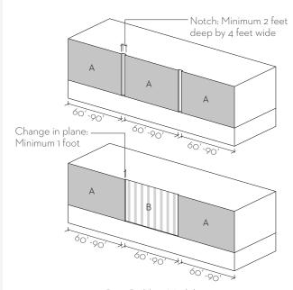
FIGURE 7.2.1 - Base Building Modulation
