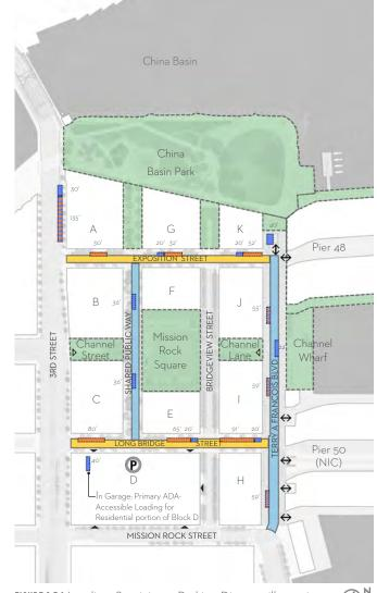
**FIGURE 2.5.1** Loading, Servicing, + Parking Diagram illustrating passenger and commercial loading locations and dimensions, shared streets, and large vehicle access points in the public realm. Loading dimensions are noted in italics next to each zone. Refer to Infrastructure Plan and Transportation Plan for more information.
