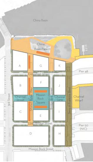
**FIGURE 2.6.1** Conceptual Paving Zones diagram illustrating the relationships among paving zones defined in Guideline 2.6.4. Paving details and conformance with City standards are defined in the Infrastructure Plan.
