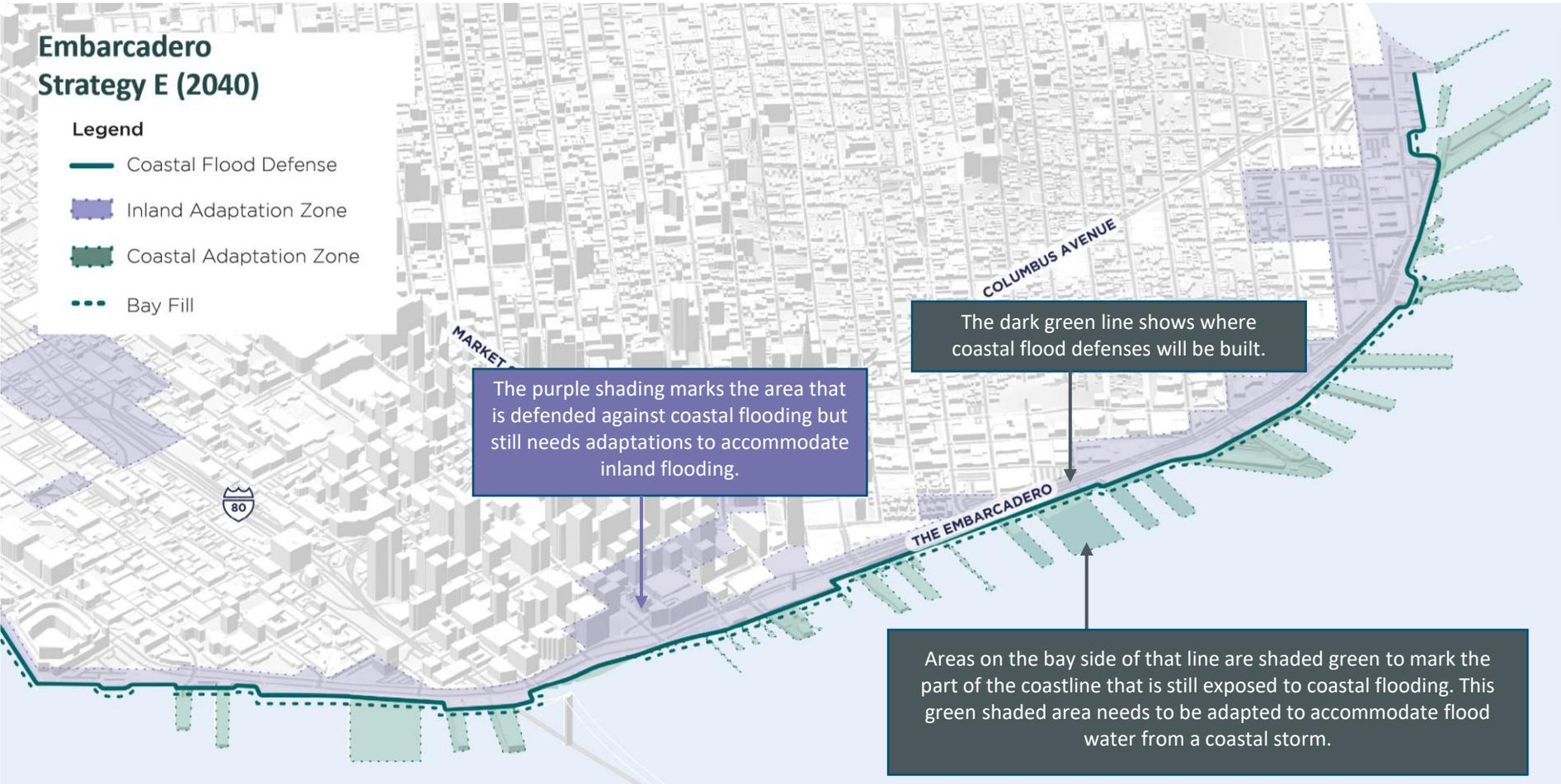
The purple shading marks the area that is defended against coastal flooding but still needs adaptations to accommodate inland flooding.
