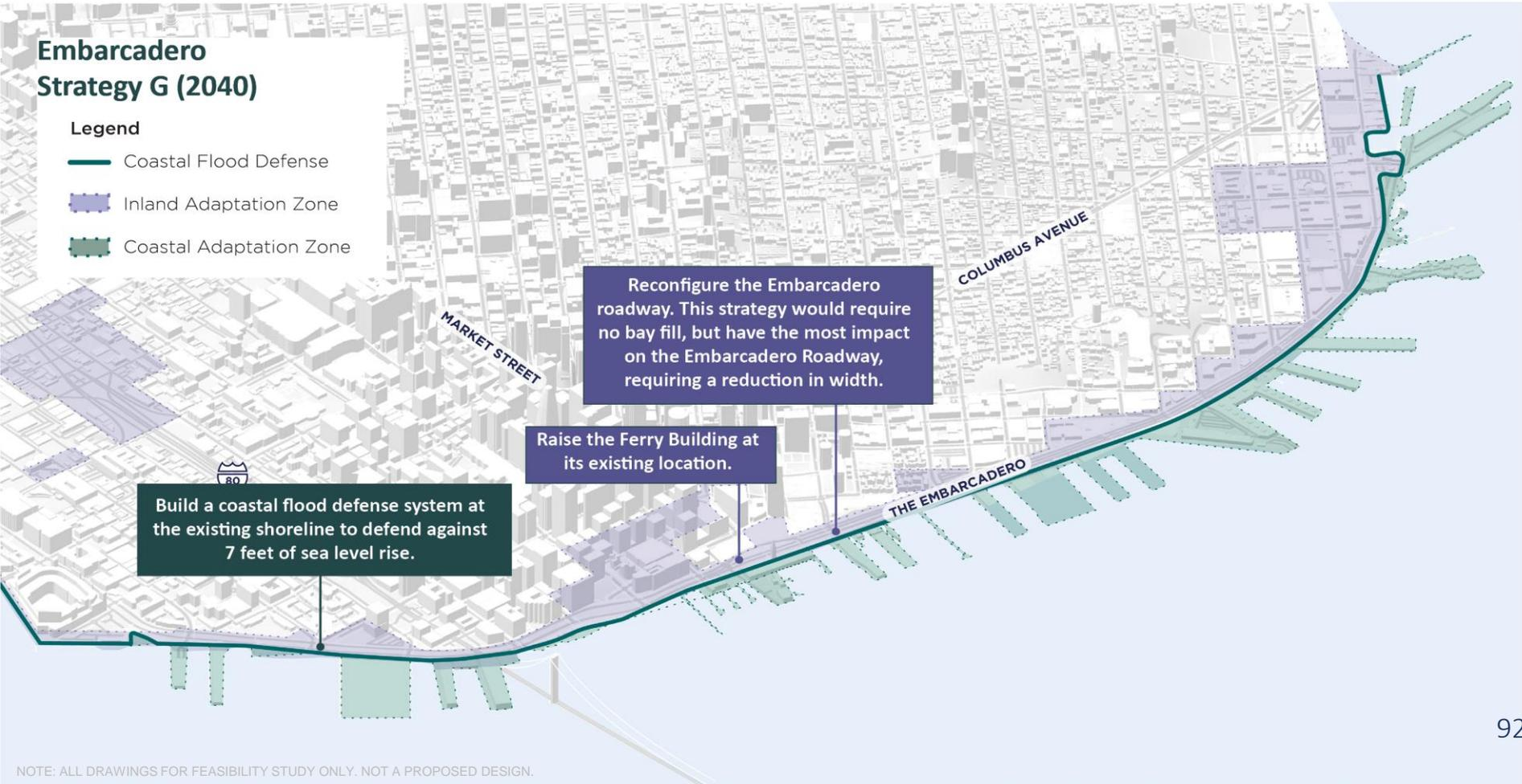
Reconfigure the Embarcadero roadway. This strategy would require no bay fill, but have the most impact on the Embarcadero Roadway, requiring a reduction in width.
