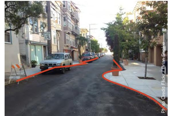
FIGURE 4.6.2: Example of Bulb-outs, Chicanes, and On-Street Parking
