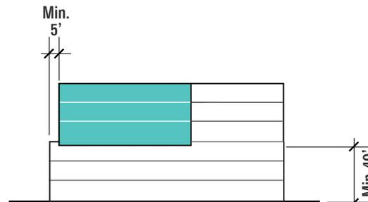
Partial Floorplate Horizontal Building Connector - Section
