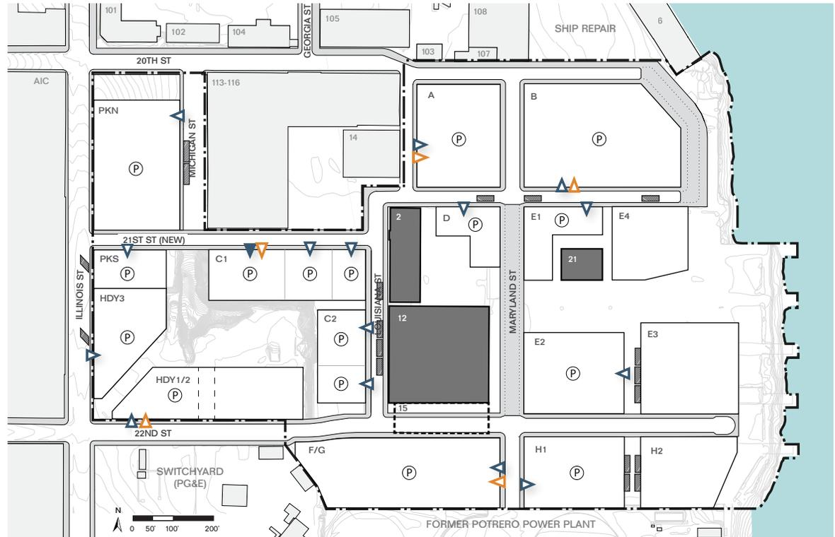
**FIGURE 5.6.2:** Illustrative Plan of Loading and Parking Access
