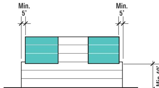
Horizontal Building Connector with Central Opening to Sky - Section
