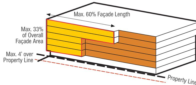
**FIGURE 6.10.3:** Aggregated Occupiable Projections
