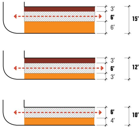
**FIGURE 4.3.3:** Effective Sidewalk Width – 6' Minimum Throughway Zone
