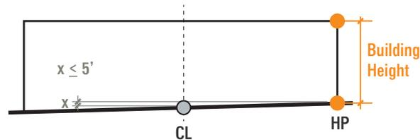
If the difference between High Point (HP) and Center Line (CL) is equal to or less than five feet
