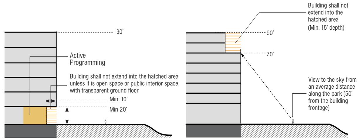
**FIGURE 6.19.4:** Ground Floor and Upper Level Setback Requirements
