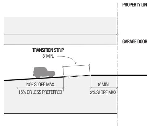
**FIGURE 5.6.3:** Driveway Slope and Top Transition Strip
