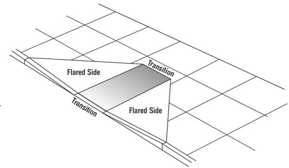
FIGURE 5.6.7: Perpendicular Curb Ramp
