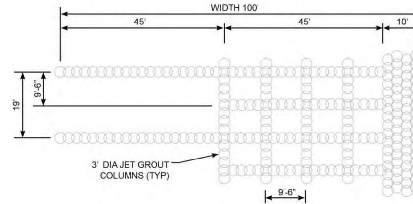
Jet Grouting - Partial Plan View
