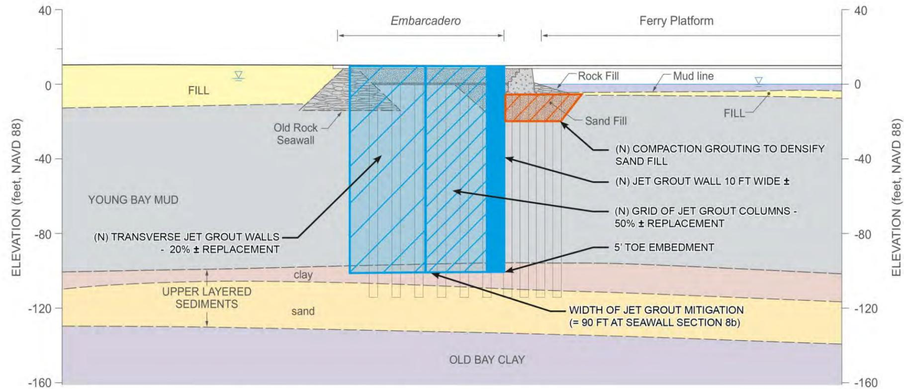
NOTE: Mitigation concept requires consideration of BART tunnels, SF Muni Turnback Structure, utilities, pile foundations, old rock seawall, etc.
