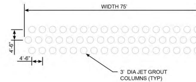
Jet Grouting - Partial Plan View
