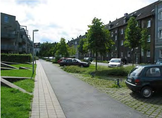
*Permeable pavers are used in parking spaces in Germany.
